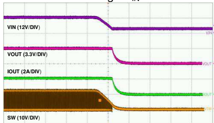
Shutdown Through V IN 2A Load
