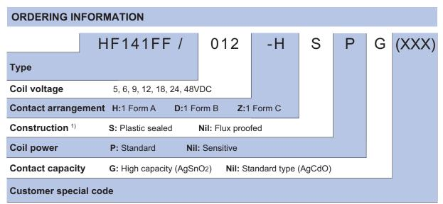
**Notes:** 1) Under the ambience with dangerous gas like H<sub>2</sub>S, SO<sub>2</sub> or NO<sub>2</sub>, plastic sealed type is recommended; Please test the relay in real applications. If the ambience allows, flux proofed type is preferentially recommended.
